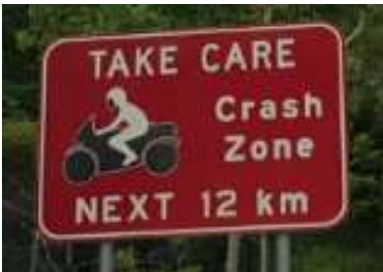
Figure 2.3.1 Example of a Motorcycle Crash Zone warning sign that could be utilised on high risk areas.
